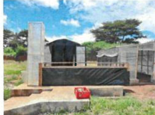
From left to right: Participants in the BSF workshop with some of the supervisors. A solar dryer built by the project is very efficient to dry the BSF larvae. This step is necessary if the larvae are to be further processed. The participants of the workshop test the solar dryer with some BSF larvae.
