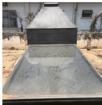
Indirect improved solar dryer
