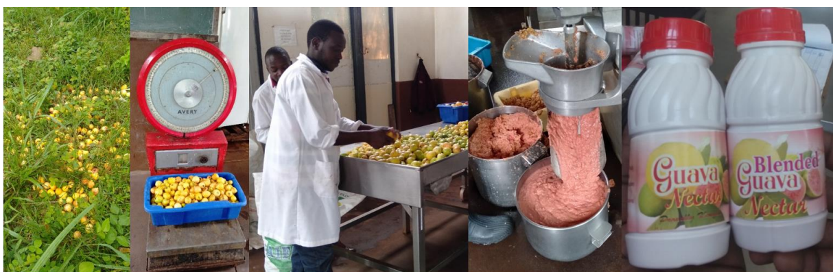
Guava surplus production, sorting, cleaning, processing and ready blended guava nectar at University of Nairobi, Kenya © D.Gekonge
