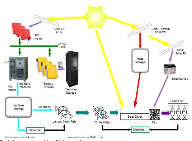
Fig. 2: System concept (simplified version)
